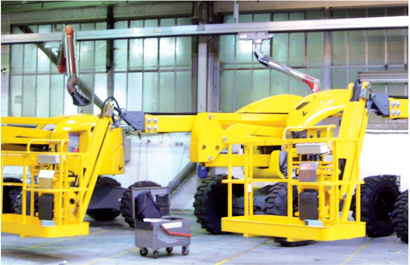
BRAS ARTICULÉS SUR RAIL POUR ASPIRATION SUR NACELLES/FLEXIBLE ARM ON RAIL ON CARRIAGE
